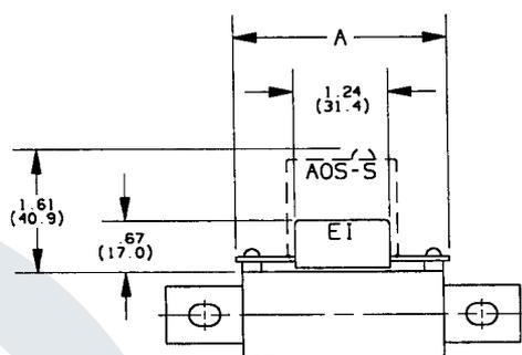
Note: Fuses with the EI option are designed to work with the AOS-S or AOS-Q add-on switch, which is ordered separately. See page J6 for details.
